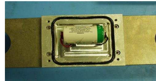
***Do not use a power drill or power screwdriver to remove or tighten the bolts – this may damage the threads on the aluminum plate.***
